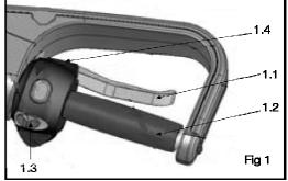
several reasons for this to be fitted. 1. to stop the throttle becoming pulled on accidentally causing a dangerous situation. 2. to stop intentional very rapid acceleration. 3. for emergency use. 4. it is possible that when in an emergency situation, instead of releasing the throttle some people will panic and pull the lever even harder. With this sensor fitted, in an emergency situation which ever direction the lever goes the machine will stop. In normal use take
