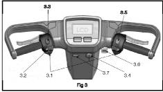
10. Forward/Reverse Switch – Located on the RH handlebar (fig 1.3). Select your desired direction by pressing either side of switch as marked. When using reverse the top speed is automatically reduced and a warning buzzer will sound. WARNING Always come to a complete stop before changing selector switch.
