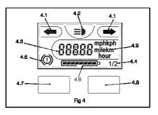
15. **Speed Indicator Display –** Located on the LCD display (fig 4.3) the Speed indicator shows the speed the Breeze is travelling in either mph or kph (fig4.9).
