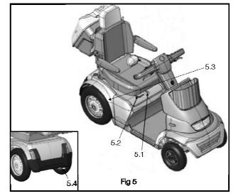
6. The seat height is adjustable by altering the position of the seat stem. Remove the seat and rear cover and you will see the seat stem is held in its location by a single bolt. Remove the bolt and the seat stem can be adjusted up or down to any one of its fixing holes. Adjust to your preferred position and tighten bolt. Refit cover and seat.
