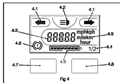
15. **Speed Indicator Display** – Located on the LCD display (fig 4.3) the Speed indicator shows the speed the Breeze is travelling in either mph or kph (fig 4.9).
