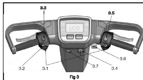
10. **Forward/Reverse Switch** – Located on the RH handlebar (fig 1.3). Select your desired direction by pressing either side of switch as marked. When using reverse the top speed is automatically reduced and a warning buzzer will sound. **WARNING** Always come to a complete stop before changing selector switch.
