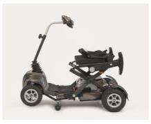
Once the tiller is clear of the seat place the other hand under the seat and continue to pull both until the Maximo is fully open as shown below. Then lift the back of the seat and rotate the arm rests forwards.
