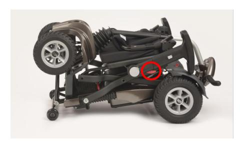
Then stand to the side of the Maximo place one hand on the tiller and lift away from the seat
