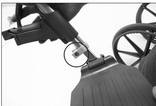
2. To adjust the footplate angle to the required position, loosen the screw located at the side of the footplate and adjust to the required angle. Tighten the screw until secure (see Fig.6).
