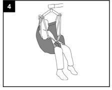
Move the hoist into position and attach the leg straps to the hooks on the spreader bar. Next attach the shoulder straps to maintain an upright seated position as shown in the diagram above. The lift may move towards the patient as you do this. When reseating the client, use the sling positioning handles to help achieve a safe and comfortable position.
