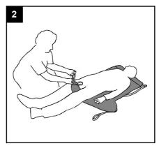
Carefully feed the leg sections under and up between the patient's legs, ensuring that the sling is positioned comfortably and not twisted or creased under the thighs. Configure the leg straps in the same manner as with the seated position (step 3). Next, proceed to attach the sling to the spreader bar in the same manner as with the seated position (step 4).
