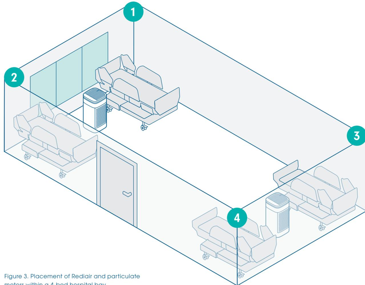
Figure 3. Placement of RediAir and particulate meters within a 4-bed hospital bay.
