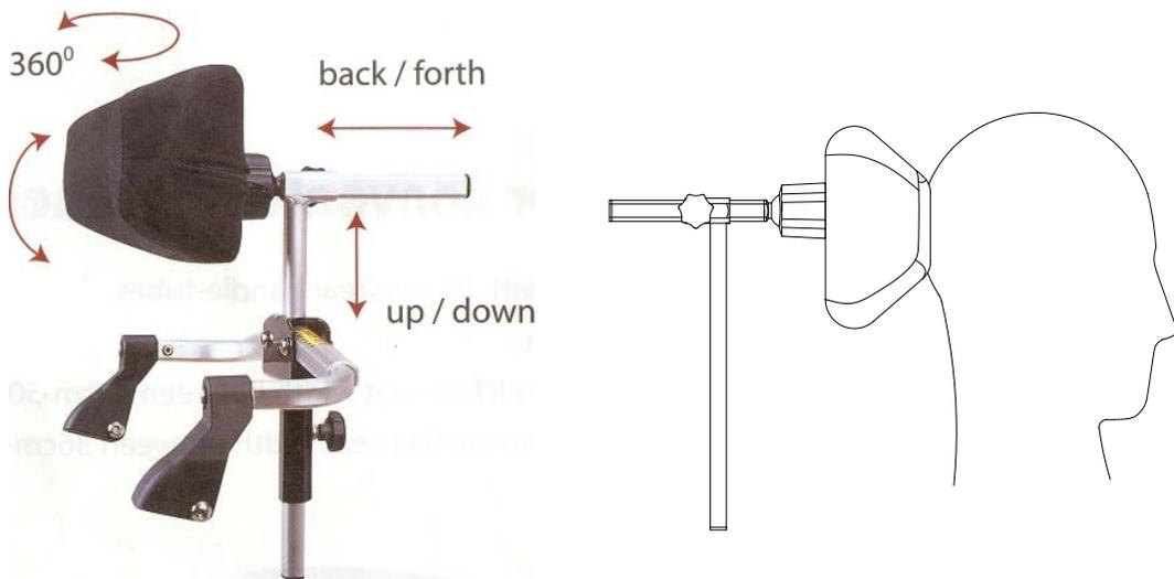
Horizontal position of headrest should be set for occupant comfort within 10mm of head. Height of headrest should be set to centre of occupant's head. The height of the headrest is set by means of a fixing knob as shown in the diagram. Release of this knob allows the cushion tube to slide up or down. When at the required height the knob should be set finger-tight. Do not overtighten.
