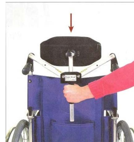
Conversely when folding wheelchair, first pull down the headrest to release the support tension, then fold wheelchair.
