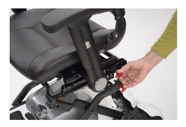
2. Slide the seat forwards slightly and lift away from the base.
