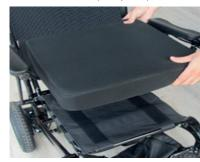
10. Charge battery. The battery can be charged via the powerchair by inserting the charger into the socket on the underside of the joystick. The battery can also be charged directly when removed from the powerchair. (See section 8.3 of the Instructions for use for more details).
