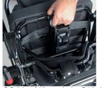
5. Switch on folding mechanism. Set the lower switch at the rear of the chair to 'I'. To fold out the powerchair, press the upper switch on the side marked 'l'. Continue to press until the powerchair is fully folded out.
