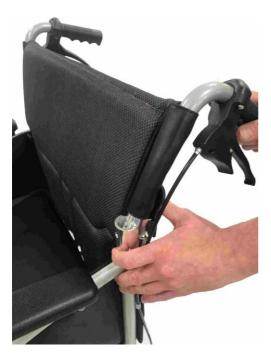
Push the black paddle towards the back post with your thumb whilst pulling the handle down, as shown. Repeat this operation for the other handle. To put the backrest back into position, lift both handles together and the folding mechanism will lock back automatically.
