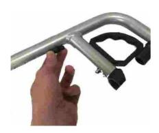
The height of the foot plate can be adjusted to suit the individual user.
