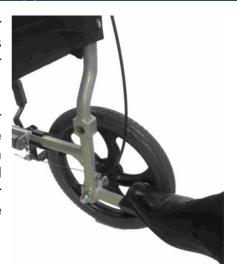
**To mount a kerb**. Approach the kerb head on. Then the attendant uses the stepper tube to raise the front castors, and lowers the front castors on the raised kerb. Finally the attendant should push the wheelchair forward, lifting it up slightly to mount the kerb if required.
