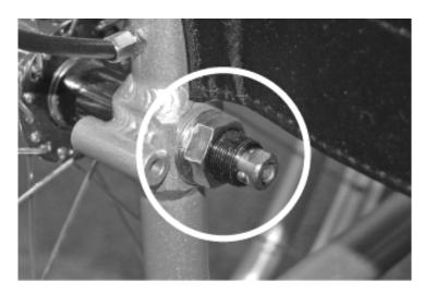
It is important that the quick release wheel axle is inspected and maintained at least monthly.
