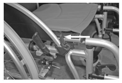
For easier side transfers, the armrests can be flipped backwards. Simply press the lever arrowed opposite to the and lift the arm back out of the way. To fully remove the arm, turn the lug at the back of the arm and lift the arm assembly clear of the wheelchair.
