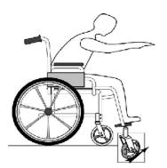
DO NOT sit on the front of the seat and attempt to reach for high objects. This could potentially lead to a forward tip and injury to the user.
