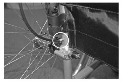
It is possible that after some time there may be a small amount of stretch in the cable. The stretch can be compensated for by using the adjustment screw as shown opposite. It uses the same principle as that of a bicycle brake.
