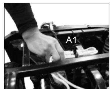
**CAUTION:** Take into account the heavy weight of the batteries (C1) please consider your physical condition before disassembling. **DO NOT** short-circuit battery connector (C1). The red wire on the battery connects to the red positive location, and the black wire to the black negative location. For safety, please wash your hands after disassembly.
