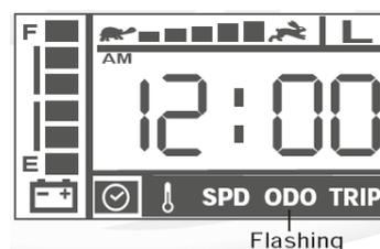
**2. Display II for Routine Maintenance** - After the routine maintenance is finished, the user could setup the mileage for next maintenance. (Count down setting) Setup steps:
