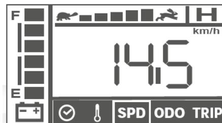
When "km/h" is displayed, speed will be indicated in km per hour. When "MPH" is displayed, speed will be indicated in miles per hour. When "/h" is displayed, the function of speedometer will be disable. (This display will be applied to the model that is not equipped with optical coupler) And the display will be replaced to WIP (accelerator) operation indicator as follows:
