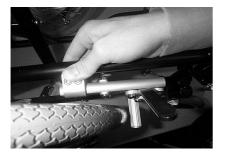
Retighten the brake clamp screws using the supplied allen key to secure the brake unit in position
