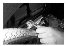
3 Remove the existing brake unit as shown below:
