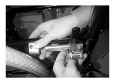
4 Replace with the Easibrake brake unit and position the brake unit in the desired place as shown below:
