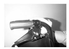
9 Using the screw, washer and nut; clamp together the brake handle and bracket using the supplied allen key to secure.
