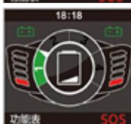
5. When the power is lower than 10%, Battery widget is red, showing that do not allow to move, the power is too low, the scooter will automatic shutdown a few minutes later.
