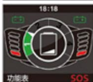
2. When the power is lower than 10%, Battery widget is red, showing that do not allow to move, the power is too low, the scooter will automatic shutdown a few minutes later.
