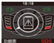
1. If the battery widget is in a red state, please charge as soon as possible, reduce the use of driving function, change to the push model. If you fail to comply with this condition, you may be trapped in an insecure location, such as a road central.
