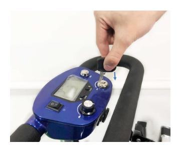
9. Secure the armrest by screwing the threaded knob into the hole (arrowed).
