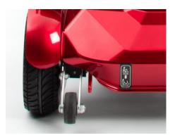
Switch off the scooter and push the lever DOWN to engage FREEWHEEL mode. This should only be engaged if you need to push the scooter manually. Do not sit on the scooter whilst in freewheel mode as this could cause damage and/or injury. The scooter will be hard to manoeuvre if left switched on.
