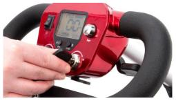
Step 2: Press the A-Open button on the control panel for 5 seconds and then release it. The buzzer will sound continuously, indicating that the control is ready to pair to the key fob.
