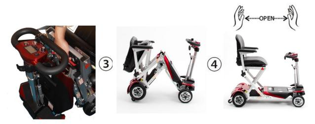
Note: You can fold or unfold the scooter manually by releasing the red manual fold release lever. If this is performed, then the opposite action should also be performed manually to reset. Failure to do so will not damage the scooter, but the auto-fold function may not work until the folding mechanism is manually reset. For this reason, it is recommended the manual operation is performed in emergency only.
