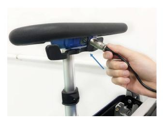
3. Insert the key into the ignition (as shown below) and switch the scooter on. Then press button on the tiller dash marked 'A-OPEN'. The scooter will then slowly beep and unfold. For safety, the unfold process will stop halfway. Press the button again to fully unfolded the scooter. When fully unfolded the scooter will emit three quick beeps.
