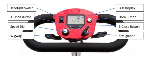
The AutoFold Elite Scooter features an LCD display (below). The Speedo shows the current speed of the scooter. The Power Gauge shows battery voltage and remaining power in the battery. The Odometer displays the current travel time and mileage.
