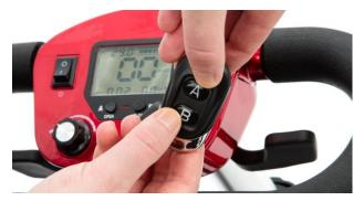
Step 4: Press the B-Closed button on the control panel to silence the buzzer and complete the pairing sequence.
