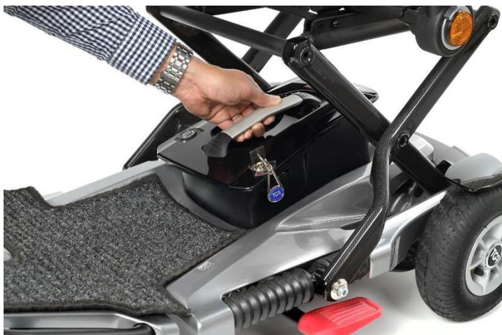
To remove the battery pack first ensure the pack is unlocked by inserting the key into the pack and turning it 90° anti clockwise to the unlock position. Then simply lift the pack up away from the base of the scooter and the seat using the handle provided.
