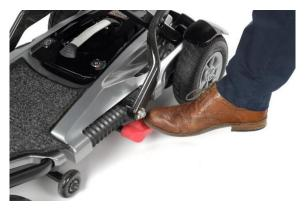
4. Once folded you can then lift your scooter using the handle at the rear and stand it on its front wheels to move around in the folded position.
