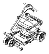
3) Lock the scooter onto the open position by pulling the seat up and pushing the tiller forward until a click sound is heard.
