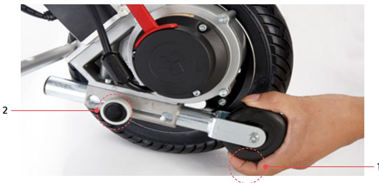
1. As shown in Fig. G1, press the anti-tipping wheel button. Pull out the anti-tipping wheel to the position of the hole for it to lock.
