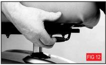
Caution: Test that the seat has fully locked by hitching backwards and forwards.
