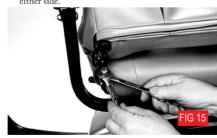
Warning: Both stop bolts must be positioned in the same position for the backrest to be fully supported, failure to observe this warning may distort the backrest frame.
