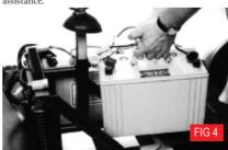
5. Secure the two batteries into position with the clamp bracket T bolt (Fig 5) and wing nut supplied (Figs 6). Note: The 'J' bolt hooks into an 8mm hole situated in the seat post support bracket.
