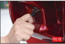
The handlebar lock is operated by a black lever positioned handlebar (see Fig 18). To release the handlebar from a locked position pull the black lever upwards, the handlebar will now move freely, but under mild tension.
