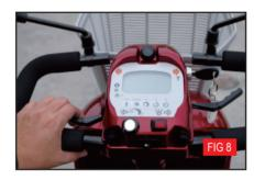
Warning: Do not attempt to operate the right and left lever simultaneously, failure to observe this warning may distort the lever system and could put you at risk. It should also be noted that reverse speed is set at half of full speed, this is a safety precaution, always make certain the Hi/Lo speed switch and the 'min and max' speed selection dial are set high enough to give you adequate power for your reverse maneuver.
