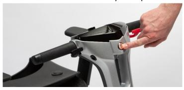
6. Once your journey is complete, Repeat step 2 and unfold the scooter. Slide the battery pack in to the scooter. Remove the Travel Cable.
