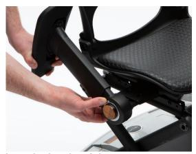
10. Adjust the height of the armrests to suit the user, by pressing the button underneath the armpad whilst lifting up the armpad.
