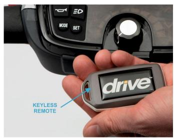
**Power.** The scooter will only operate when the keyless remote is near. To start up the scooter, hold the keyless remote near the scooter and keep the remote within 1 metre (3 feet) of the tiller dash.
