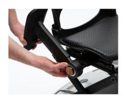
**Handlebar Height Adjustment.** Turn the large adjustment knob on the front of the tiller anticlockwise to release the handlebar. Slide the handlebar to the required position, then turn the knob clockwise to secure the handlebar in place.
