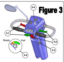
1. Set the Breeze Midi speed to slow. Hold the Tiller with both hands and gently ease the control lever to move the Breeze Midi forward. The more you pull the lever, the faster you will go. Always come to a stop before adjusting the pre – select speed control, or forward and reverse.
