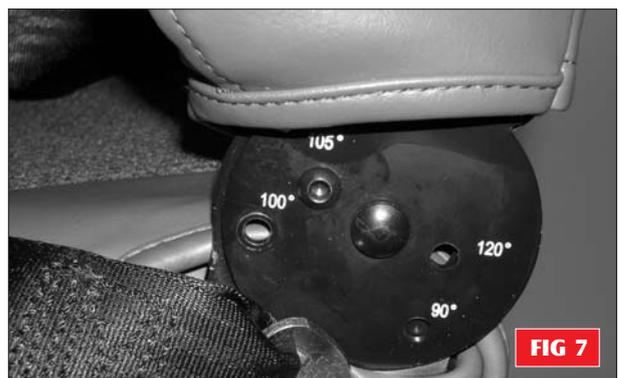
take great care when going up steep slopes or kerbs, always lean forward to achieve the best stability for your Scooter. **Do not drive up a slope greater than 5° if your backrest is positioned at the 120° position. Failure to observe this warning may put you in a dangerous situation.**
