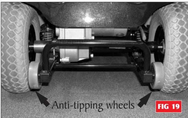
Always have the anti-tipping wheels fitted to your Scooter (Fig 19) .They are an important part of your Scooters design and reduce the likely hood of backward tipping.
