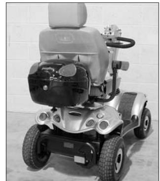
**Warning:** The rear basket and crutch/cane holder will extend the dimensions of your Scooter. Please allow for this when turning. Do not overload carrying accessories as this will make your Scooter less stable.
